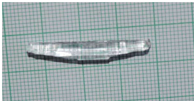
Figure 2. Photograph of as grown LAM single crystal
